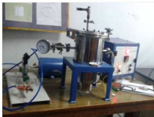
Fig.4 The MWCNTs coated glass substrate was placed inside the Gas sensing unit. The fabricated device is exposed to different concentrations of Oxygen gas. The change in the resistance was observed and the sensitivity of the device was calculated.
